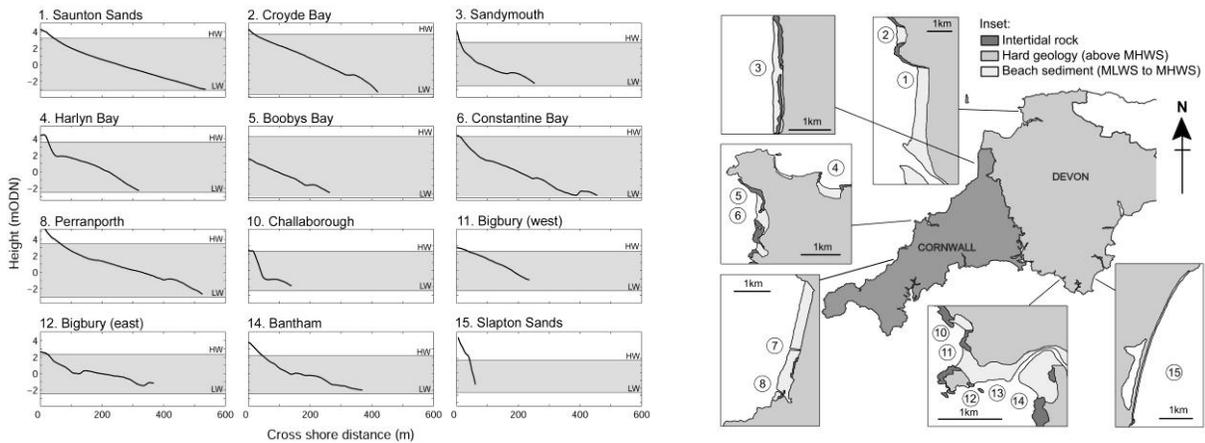
**Figure 5:** Summary of cross shore profiles and tide ranges at selected locations around Devon and Cornwall (height measured in meters above Ordnance Datum Newlyn), and schematic plan views of each site indicating beach shape, aspect of the coast and intertidal geology.
